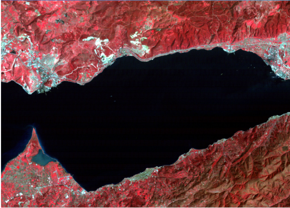
Image 8: This image shows the area on 27 March 1999. It is a false color composite of 4, 3, 2 TM bands.
