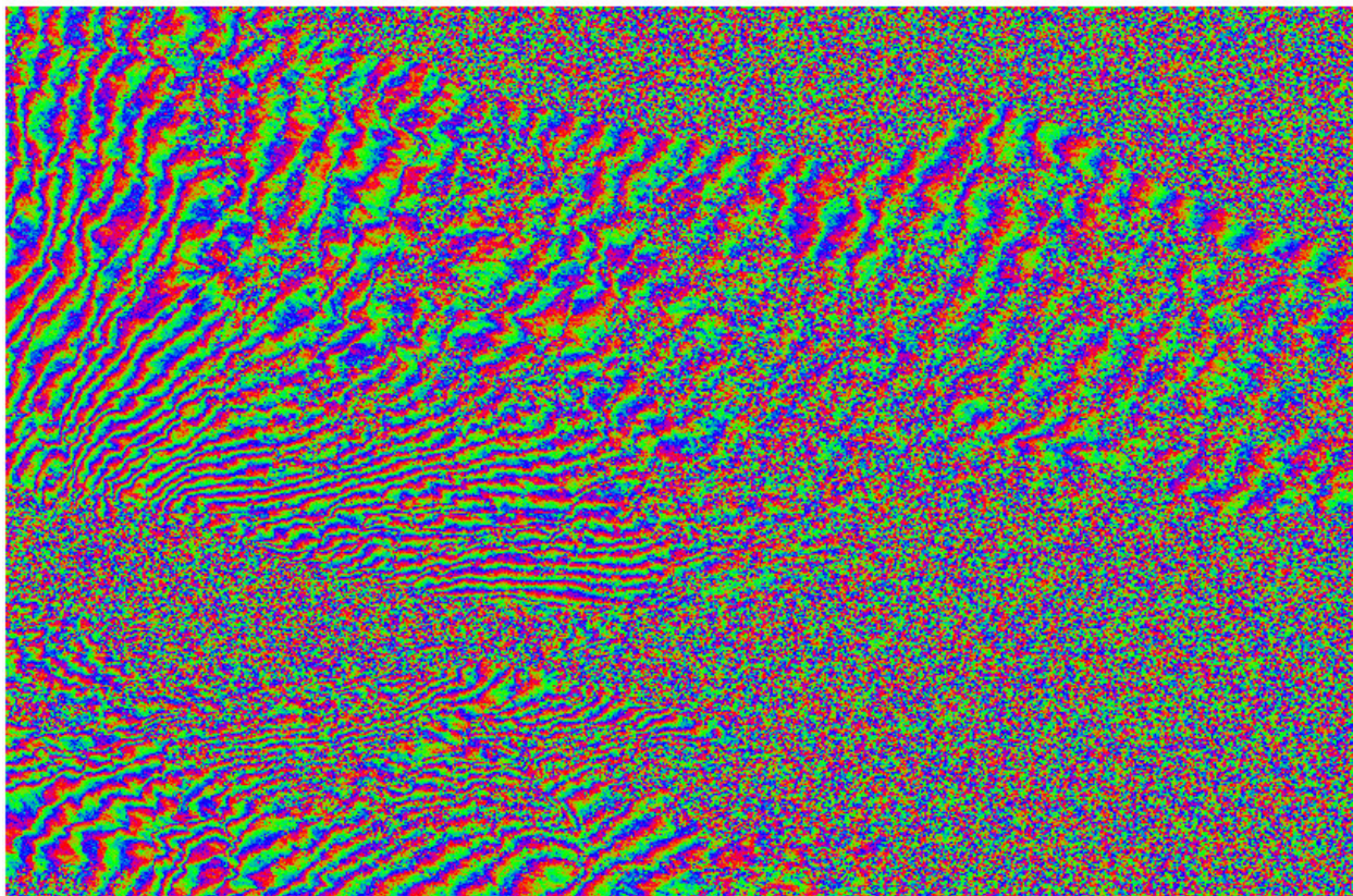
Image 28: Top image is the coherence image generated from the SLCI ERS-SAR images of 12 August 1999 and 16 September 1999. The bottom image is the phase image generated from the same image pairs.
