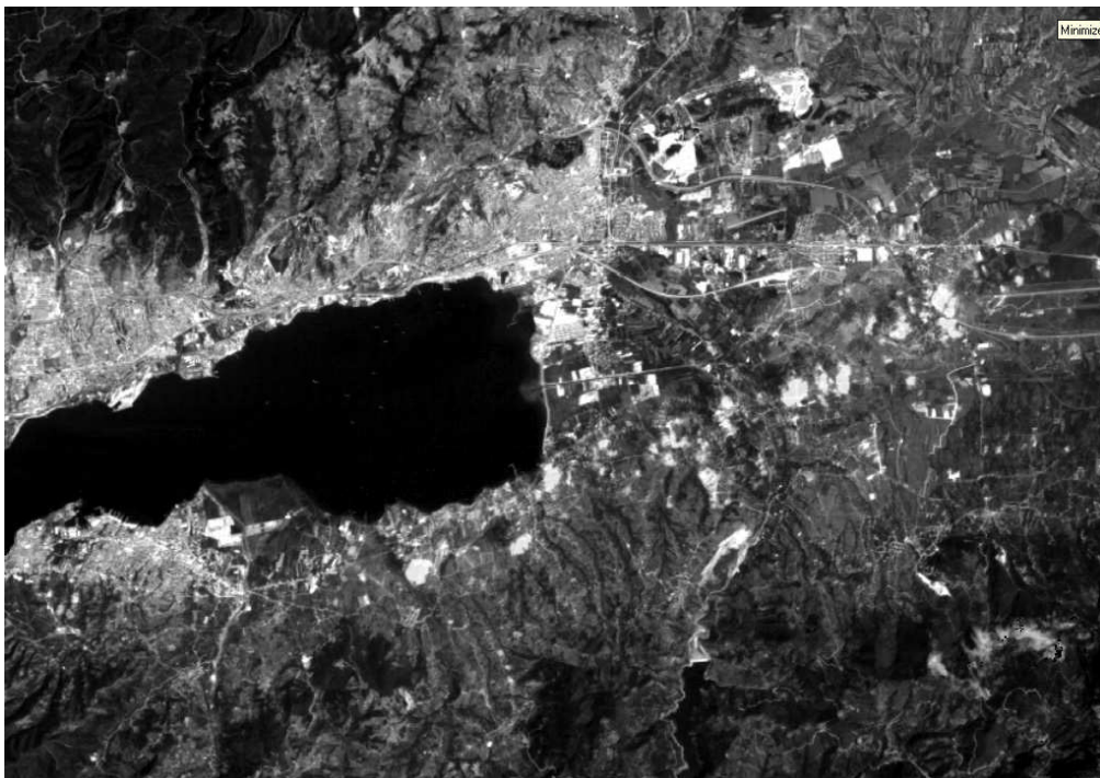
Image 11: This image shows the second principal component obtained from the integration of the band 3 of both Landsat TM images of 27 March and 18 August 1999. The second principal component image basically indicates the areas that have changed due to the earthquake. The degree of brightness refers to the rate of the change.
